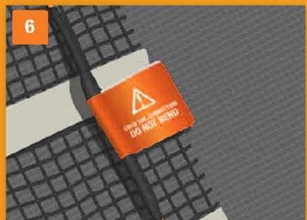
6 Take care to ensure both sections of each mat with orange warnings are laid flat on your floor.
