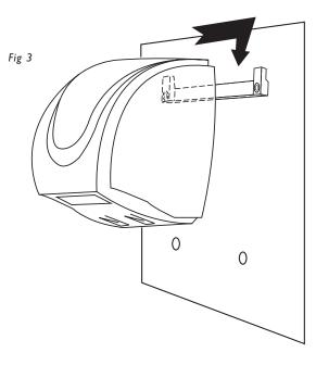
• and securing it at the bottom using the fixings provided (see fig 4).
