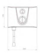
Outer Casing Easy clean, high impact Polycarbonate/ABS
