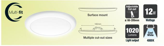
This ultra-thin (15.5mm) downlight is supplied with configurable brackets and clips allowing for installation in a cut-out from 65-160mm as well as having a surface mount installation option. Visible flicker is eliminated with the integrated driver and a frosted diffuser provides uniform light.
